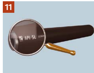
11 Final visual inspection marking ends protect
