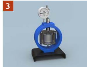
3 Tests to define resistance to sulfide stress-corrosion cracking
