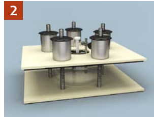
2 HIC tests to define resistance to hydrogen-stress cracking
